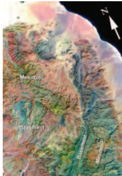
Geologically useful ASTER image of the Danakil Block in Eritrea/Ethiopia, showing Mesozoic and Recent sedimentary aquifers and crystalline basement (Steve Drury)
