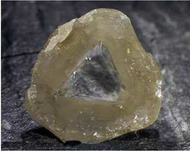
Diamond with a gem-quality core and fluid-rich "coat". The coat contains millions of tiny fluid inclusions that trap pristine brine from 200 km depth.
